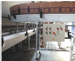
Automated batch packaging area. The system consists of corrugated box molders and sealers, conveyors, and print and apply labelers.
