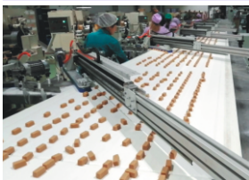
The conveyor system for homogenous distribution of sweets among 5 wrapping machines.
