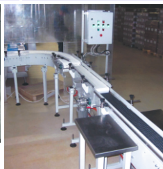
Automated batch packaging area. The system consists of corrugated box molders and sealers, conveyors, and print and apply labelers.
