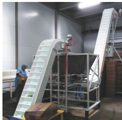
The elevator for moving confectionery products to the batch packaging area.
