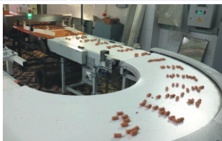
The conveyor system for homogenous distribution of sweets among 5 wrapping machines.
