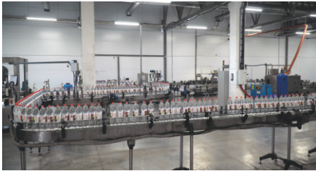
Pneumatic conveyor for transporting pet-bottles from the blowing machine to the bottling machine
