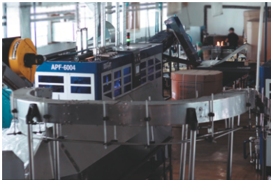
Pneumatic conveyor for transporting pet-bottles from the blowing machine to the bottling machine
