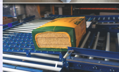
Conveyor system for consolidating product flows and moving pallets
