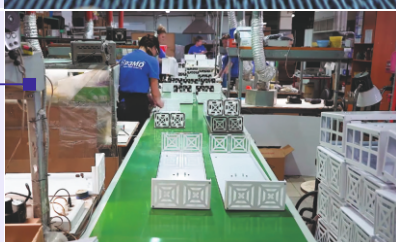
Belt conveyors for air circulation unit assembly
