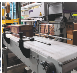
Automated batch packaging area. The system consists of corrugated box molders and sealers, conveyors, and print and apply labelers.
