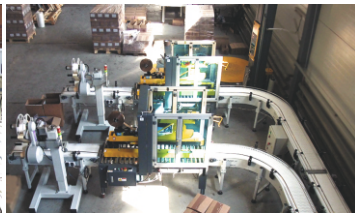
Automated batch packaging area. The system consists of corrugated box molders and sealers, conveyors, and print and apply labelers.
