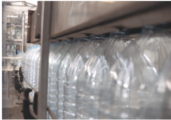
Pneumatic conveyor for transporting pet-bottles from the blowing machine to the bottling machine
